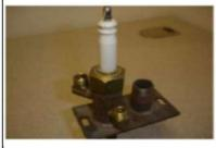
This was the original gas pilot assembly (made of steel). This gas pilot ignitor is no longer available. Therefore, you will need to order the following pilot assembly:
